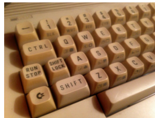
Figure 2. A photo of the Commodore 64c keyboard showing the layout of PETSCII graphics on the keyboard keys. © Raquel Meyers, 2012. Used with permission.
